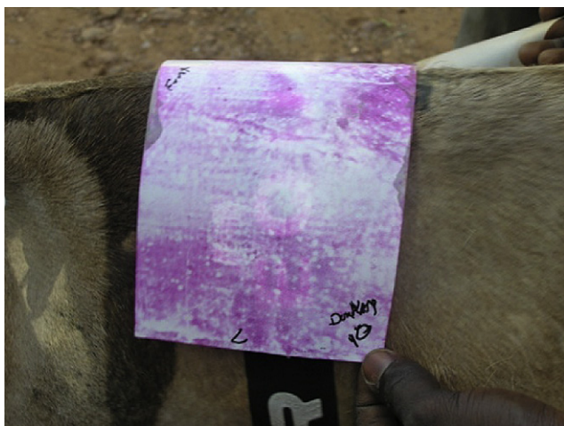
Figure 4 Extreme low pressure 4 LW Fujifilm showing low-intensity results. This film was used with a good cart and harness. The film shows very little pink coloration. The pink color is a response to pressure placed on the film. The less pink indicates less pressure placed on the withers and back of the donkey. This film sample is from a donkey equipped with good harness and a good cart.
